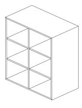
Linoleum on all outside surfaces. The edges are being produced with WO's patented linoleum edge.
